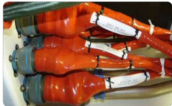
[그림 2-110] Wire harness with protective jacket
