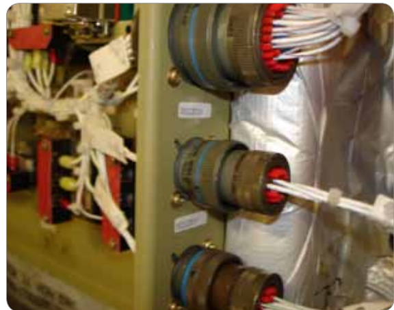
[그림 2-148] Connector arrangement to avoid wrong connection
