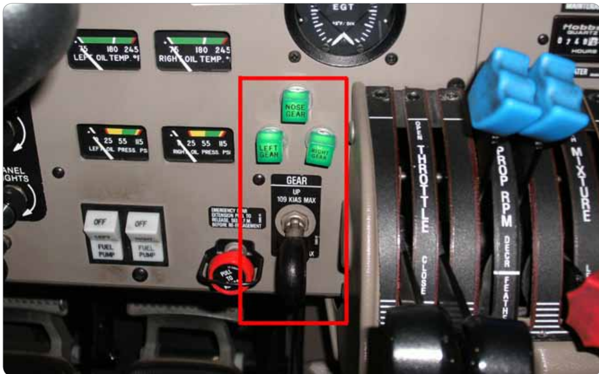
[그림 2-91] Instrument panel showing the landing gear position switch and the three gear down indicators
