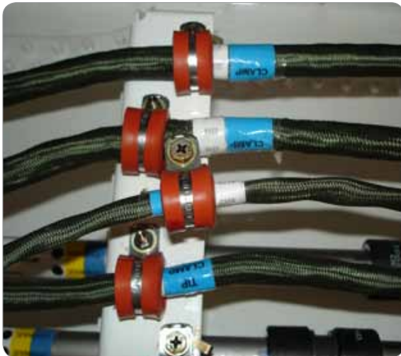
[그림 2-122] Positive separation of wire and fluid lines and wire clamps
