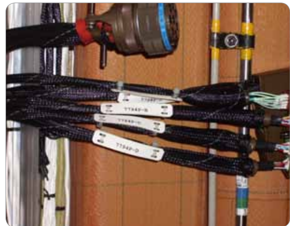
[그림 2-118] Alternate method of identifying wire bundles
