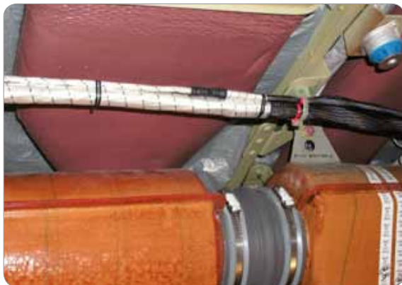
[그림 2-109] Shielded wire harness for flight control
