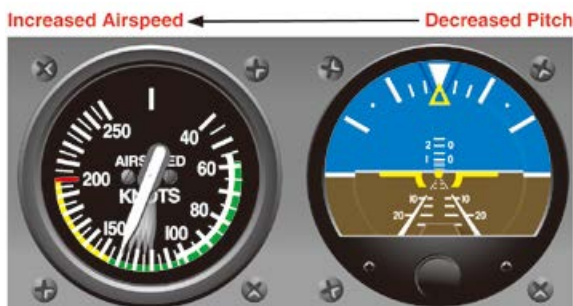
[그림 4-14] Constant power plus decreased pitch equals increased airspeed
