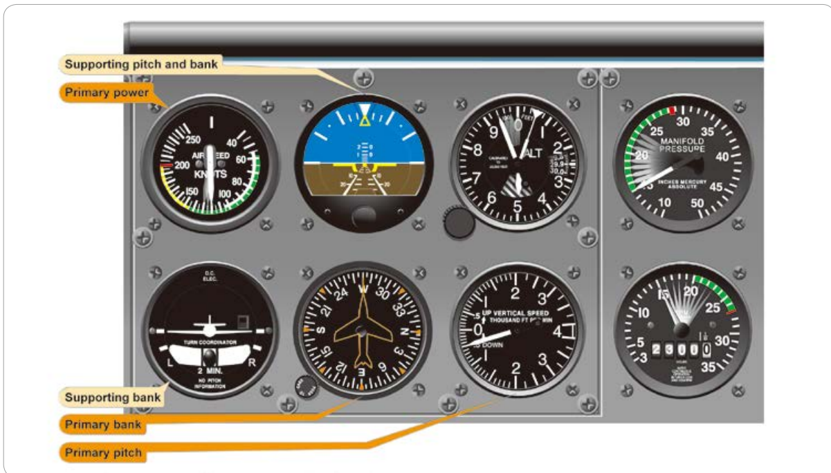
[그림 4-30] Constant airspeed descent, airspeed high—reduces power
