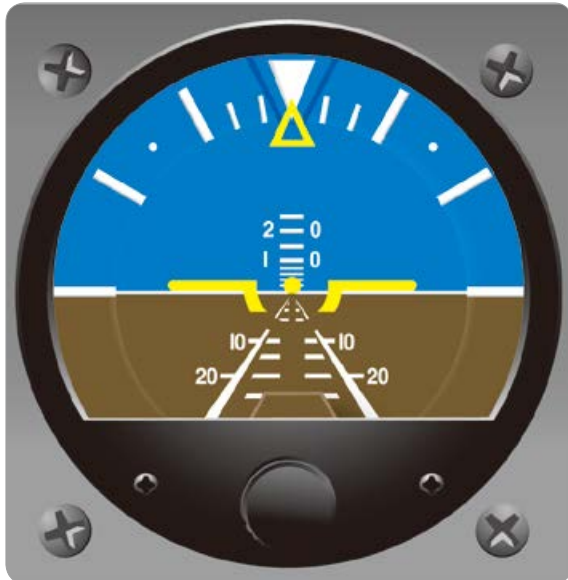
[그림 4-4] Pitch correction for level flight, half-bar width
