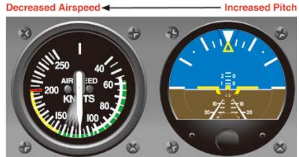
[그림 4-15] Constant power plus increased pitch equals decreased airspeed
