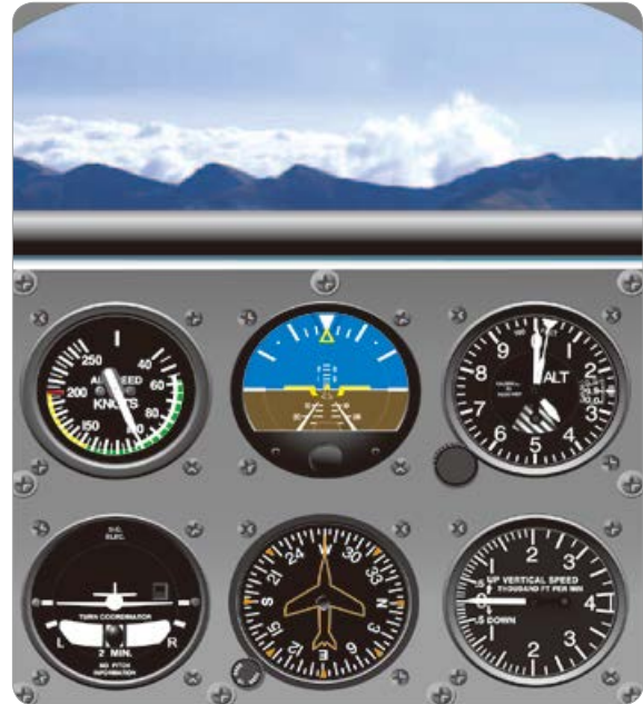
[그림 4-2] Pitch attitude and airspeed in level flight, fast cruise speed
