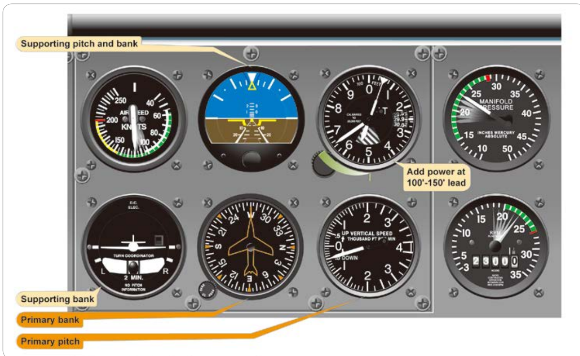
[그림 4-31] Level-off airspeed higher than descent airspeed
