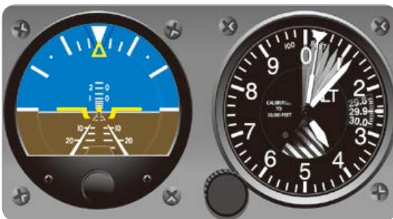
[그림 4-7] Using the altimeter for pitch interpretation, a high altitude means a nose-high pitch attitude
