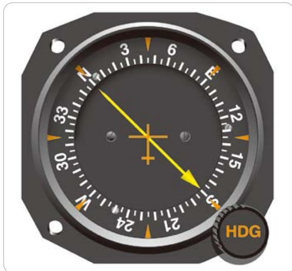
[그림 2-4] Relative bearing(RB) on a movable-card indicator
