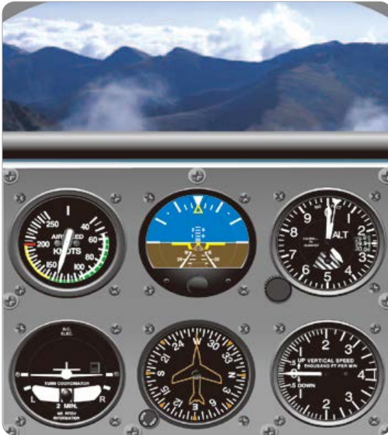
[그림 4-1] Pitch attitude and airspeed in level flight, slow cruise speed
