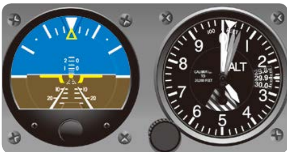
[그림 4-10] Pitch correction, less than 100 feet-1/2 bar low to correct altitude error
