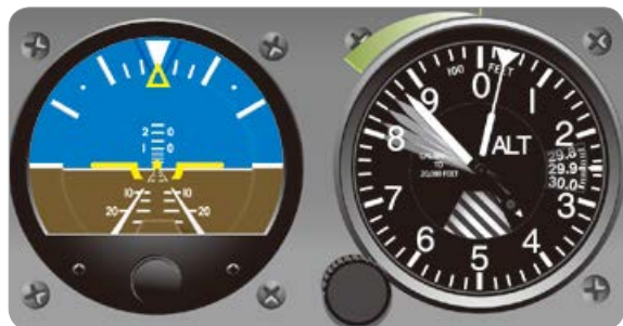
[그림 4-12] Pitch correction, greater than 100 feet-1 bar correction initially
