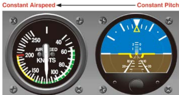
[그림 4-13] Constant power plus constant pitch equals constant airspeed
