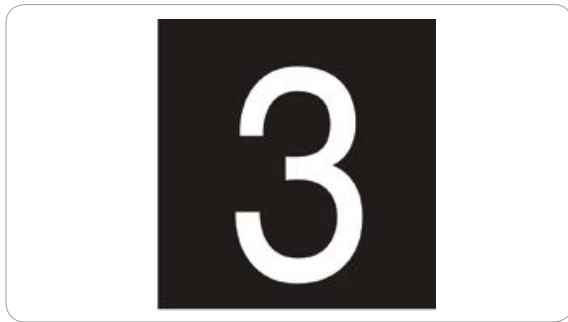
[그림 1-48] Runway Distance Remaining Sign Indicating 3,000 feet of Runway Remaining
