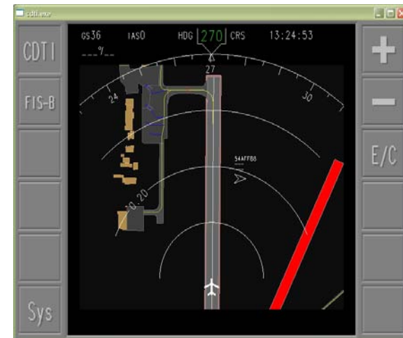
Aircraft landing on RWY 09/27 at Norrköping Airport, EFB showing RWY 11/29 Closure, from D-AIM test flight, autumn 2008
