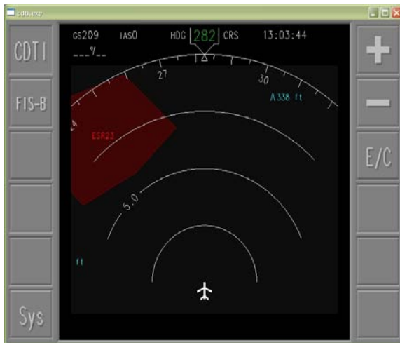
Aircraft passing activated Temporary Segregated Area (TSA), from D-AIM test flight, autumn 2008
